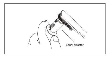
4.Check the muffler gasket; replace if damaged. Reinstall the muffler gasket, the spark arrester, the muffler and the muffler protector in the reverse order of removal.
